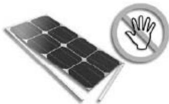
Do not apply paint or adhesive to module top surface.
